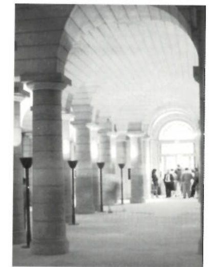
2.55. Panthéon, Paris, 1764. Jacques-Germain Soufflot. An elliptical vault with penetrations in the crypt.
